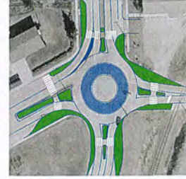
Geometric design of roundabout to be built at Bradbrooke Drive and Gladstone Avenue intersection.
